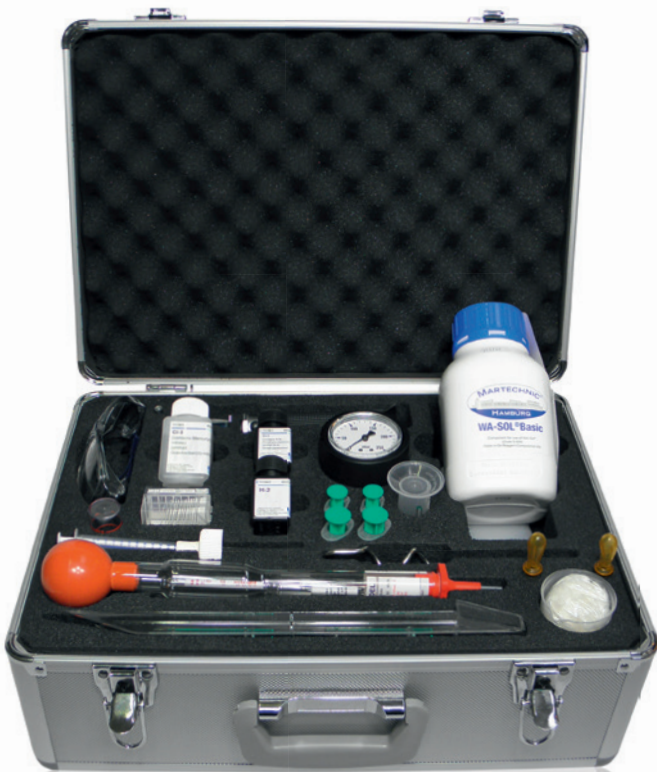
COOLANT – Customized Test Kit Example for an Emergency Generator.
